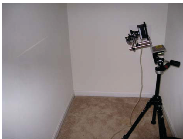
Figure 12: Setup for polarization bias measurement using line source
